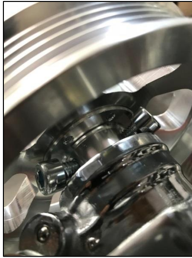
Figure 16: Power steering pulley installed with the 6mm socket head cap screws firmly tighten.
