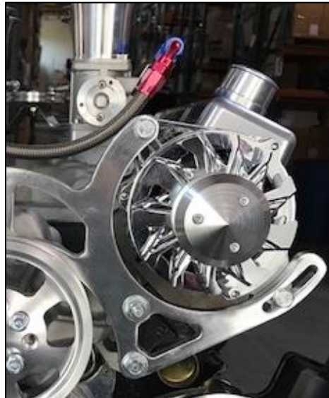
Figure 18: Mounted in the correct location of the bridge bracket.
